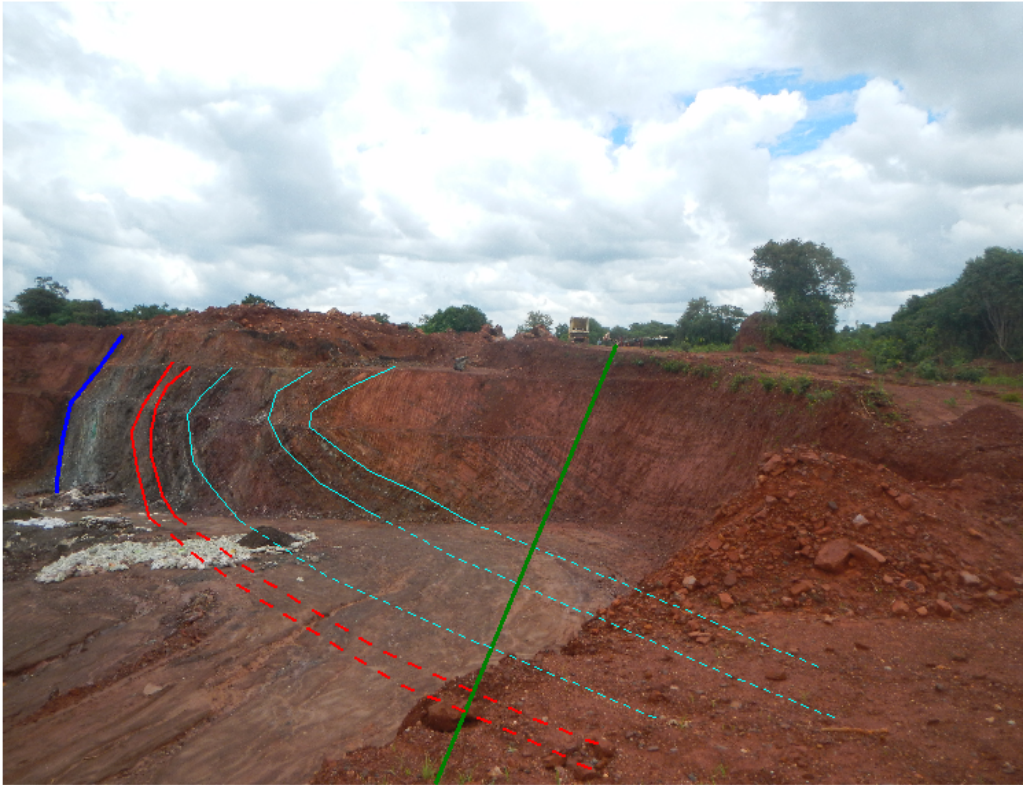
Image 1: Kasombo 5 Prospect Drill Target; shown in pit-wall of open cut; image of pit showing bedding (with light blue line, downdip projection as dotted line); basal fault (dark blue line); mineralisation target (red lines, downdip projection as dotted line); projection of drillhole (with dark green line); drill rig in position (but with its mast down) outside the rim of the pit.
