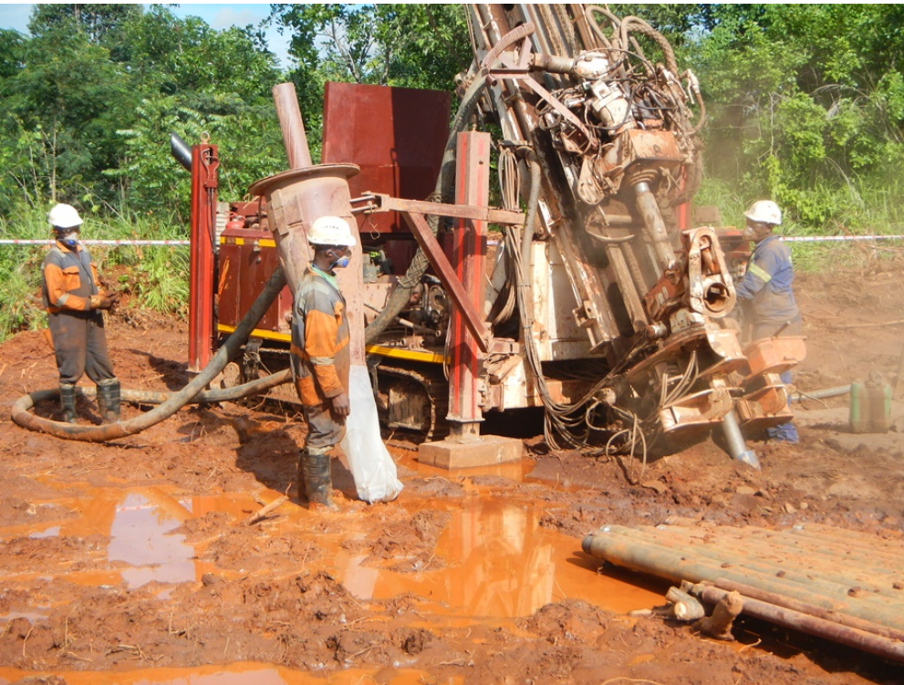
Image 2: RC drilling on a site at Kasombo 5, drillers dealing with the wet season.
