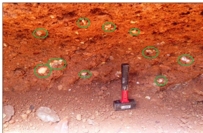
Figure 2. Alluvial gold bearing quartz fragments found in artisanal workings on the Boundiali North tenement.
