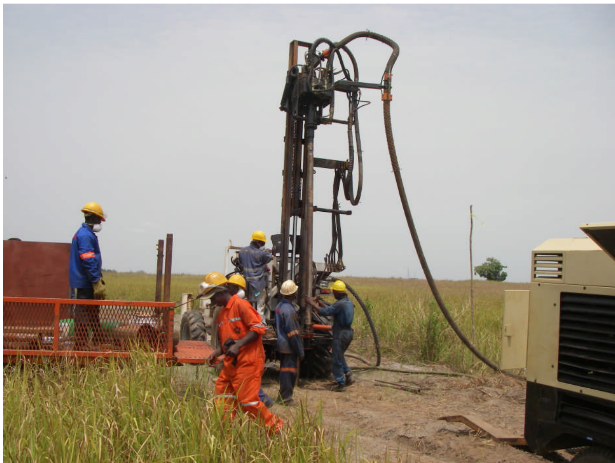
Figure 2: Air Core Drilling of Tailings at Marampa Project
