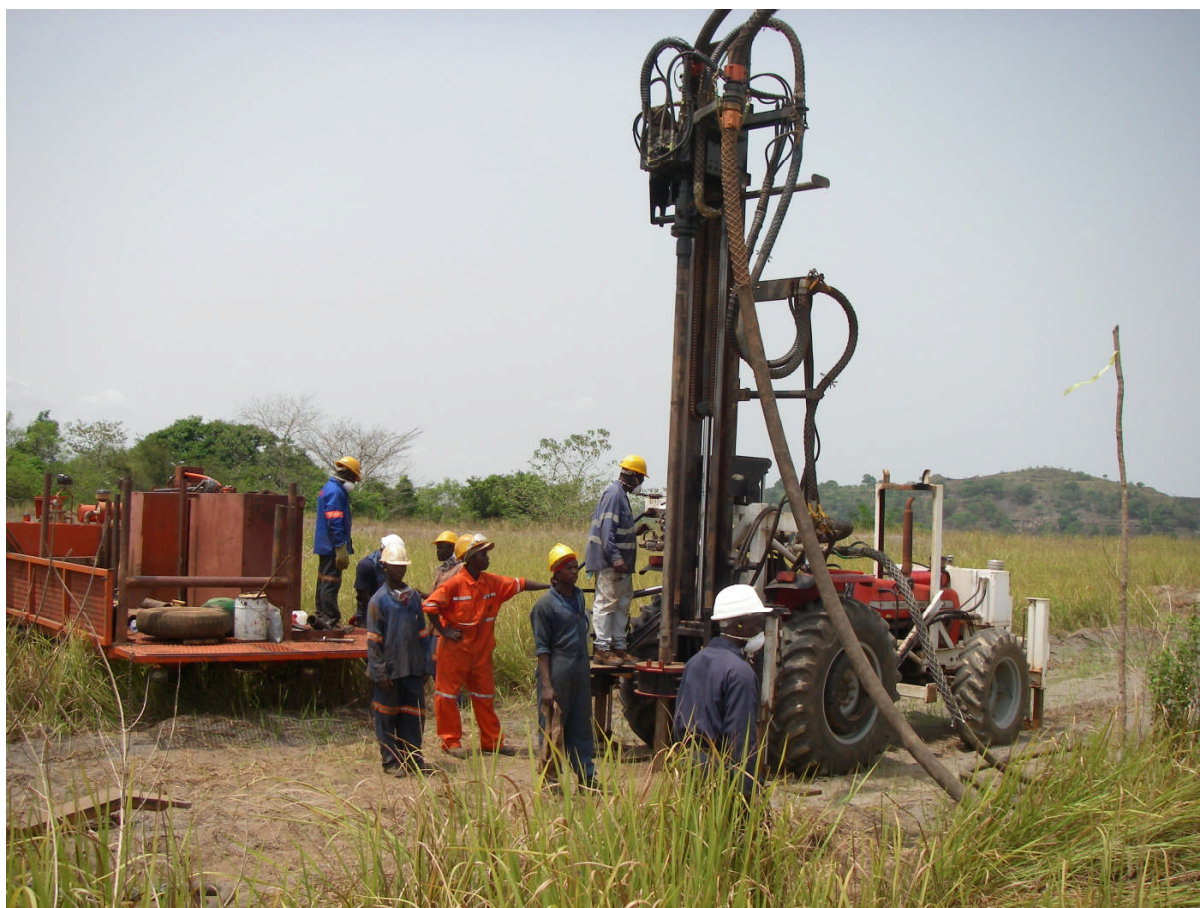
Figure 3: Air Core Drilling of Tailings at Marampa Project
